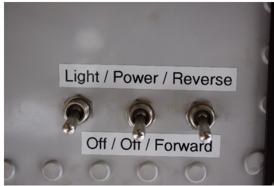
Control switches for lights, power and direction.
