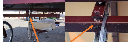
Hard to find grease zerk at rear of machine
